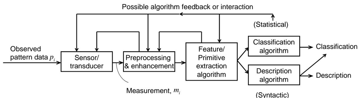
Fig. 1. Typical pattern recognition system structures
