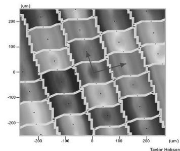
Fig. 9. Unit tile and two vectors for the tessellation for the 3M surface.
