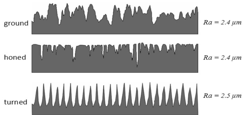
Fig. 6. Three surfaces with similar Ra.
