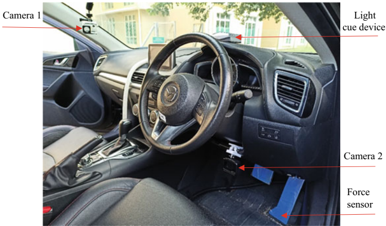
Fig. 2 Test car setup
