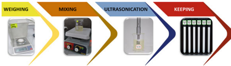
Fig. 1 Graphical process of TiO 2 -POE nanolubricants preparation using a two-step method
