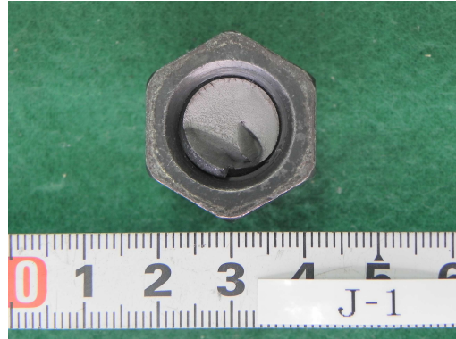
(a) \alpha=0 (fatigue life 151,860 cycles)
