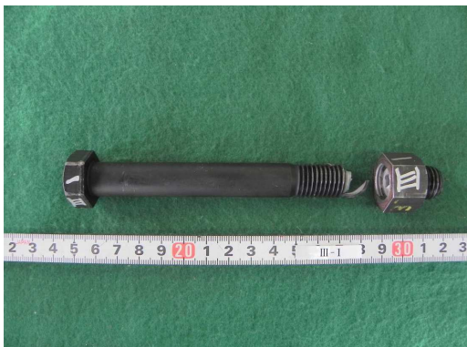
(c) \alpha=\alpha_{\text{middle}} (fatigue life 184,770 cycles)
