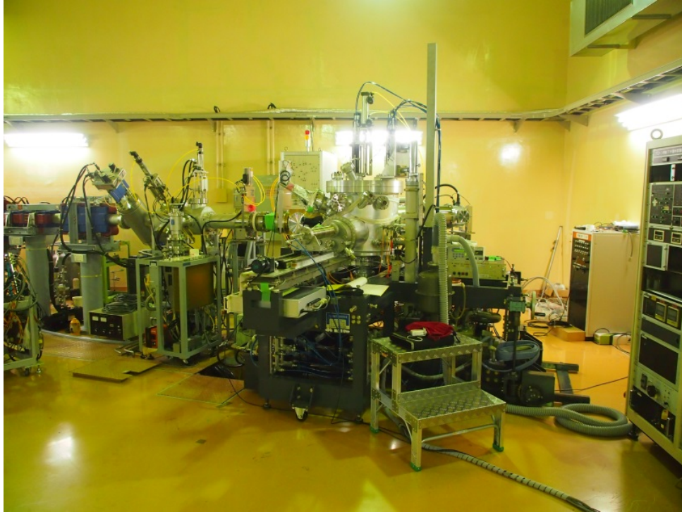
Figure 5-3. Proton Beam Line Connected to Test Chamber.
