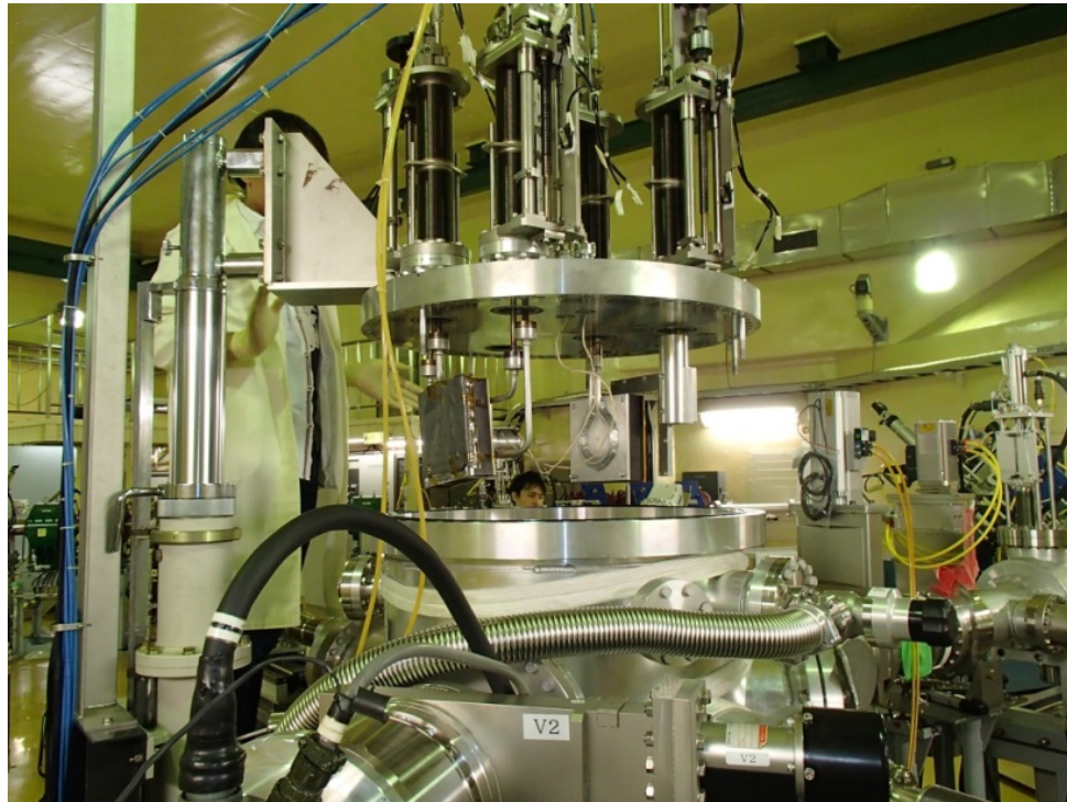
Figure 5-2. Radiation Test Chamber used in Accelerated Proton Beam Test.
