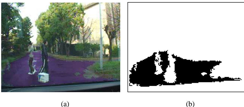
Fig. 2.6 Road region detection: (a) The result of road region detection, (b) road region template image.
