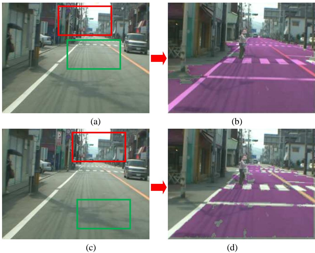
Fig. 2.13 The experiments of road region detection. (a) Training data selection, (b) the result of road region detection, (c) training data selection, (d) the result of road region detection.
