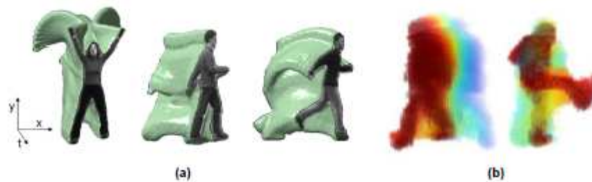
Fig. 2.1 Various motion representation schemes. (a) Space-time volume of stacked silhouettes [55, 84], (b) Motion history volumes [79]. (a) is viewed from a single camera, whereas (b) shows a recency function over reconstructed 3-D voxel models.
