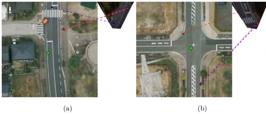
Figure 17: Examples of frames selected as outliers by global verification (Experiment 2). The dashed lines represent incorrect matches.
