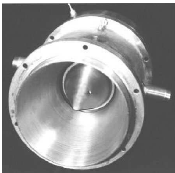
Figure 6. Photograph of the upstream part of the laboratory model showing the dominant concave outer attachment wall and the small inner convex cone.
