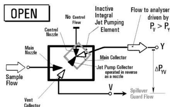
Figure 4. Schematic representation of the microfluidic valve. The flow to the analyser is driven in the 'open' state by the applied constant pressure difference  $\Delta P_{VV}$ . Its proper magnitude is regulated by turning down the 'guard' flow spilled over into the easier way out through the vent V. The jet pumping part is not active.
