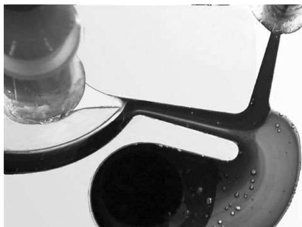
Figure 21. Scaled-up laboratory model visualization of the flows in the subdynamic phase A. The sample fluid is modelled by dark dyed water, the control flow by transparent water.
