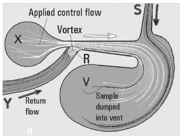
Figure 18. Computed pathlines the 'closed' state (cf. Figure 4). The powerful control flow (white lines) pushes the sample fluid from S (black lines at right) into the vent V. At the same time it generates the jet-pumping suction effect in the analyser terminal Y, creating there the desired cleaning return flow (black lines on the left).
