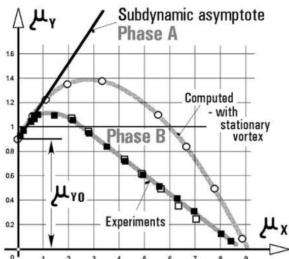
Figure 19. Flow transfer characteristic: dependence of the relative output mass flow rate  $\mu_Y$  on the relative control mass flow rate  $\mu_X$ . The switching from ‘open’ to ‘closed’ state progresses through two distinct phases, A and B.
