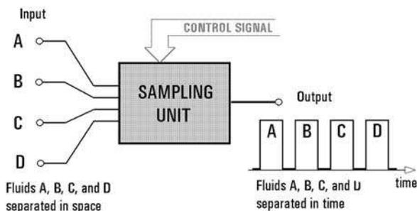
Figure 1. The developed unit essentially performs a conversion of the spatial separation between fluid samples on the input side into their temporal separation at the output.
