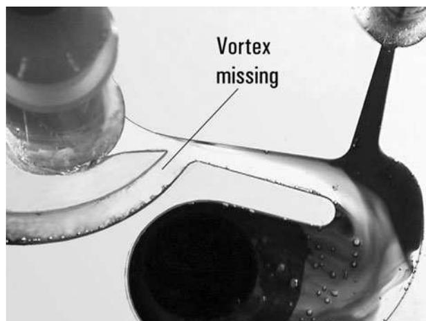
Figure 24. Visualization of the same phase B flow after some elapsed time: the vortex was shed away and with it disappeared the effect helping the control flow into the output channel.
