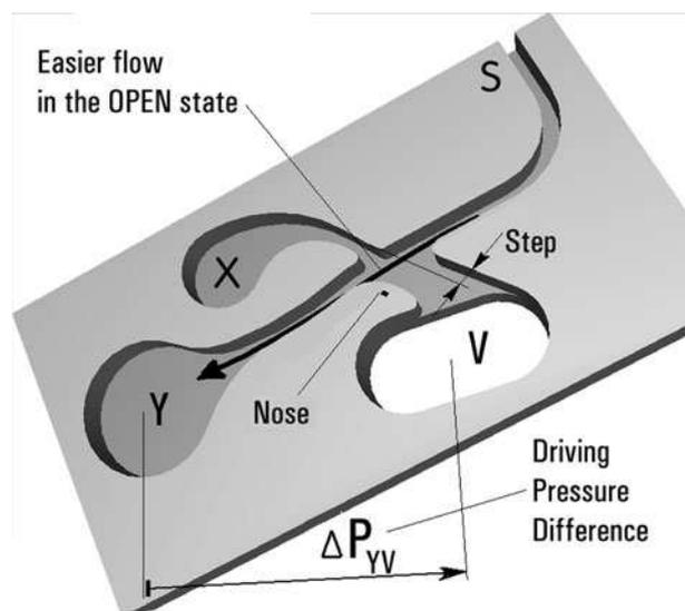
Figure 7. The first tested prototype version of the valve. To keep the driving pressure difference  $\Delta P_{YV}$  small, this version was designed with as straight as possible flow path from the reactor (located upstream from S) to the analyser (connected to V). This made the jet pump part even more rudimentary—and less effective.
