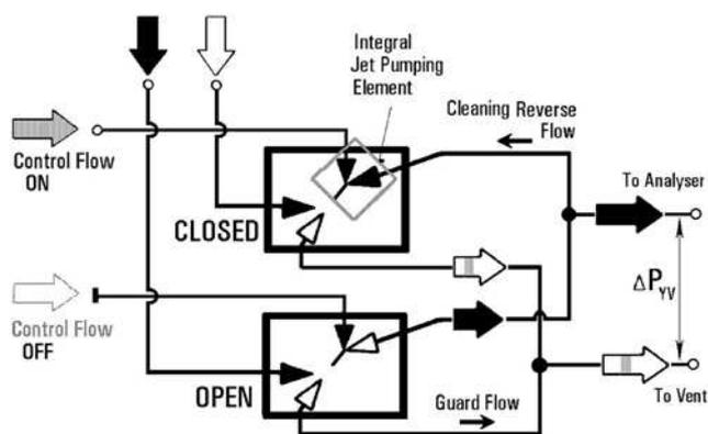
Figure 8. Schematic circuit diagram of the simplest version of the sampling unit—with only two valves, one in the ‘open’, the other, in the ‘closed’ state. The constant driving pressure difference  $\Delta P_{YV}$  is applied between the two exit terminals.
