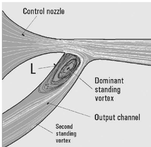
Figure 22. Computed flowfield in the phase B is dominated by the large standing vortex attached to the left wall of the output channel entrance. It the control fluid in its getting into the output channel.
