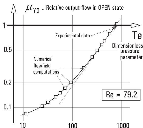
Figure 16. Diagram used to adjust the driving pressure: the relative output flow rate  $\mu_{Y0}$  (into the analyser) in the 'open' state (zero control flow) dependence on the applied driving pressure drop, plotted by means of a dimensionless pressure parameter  $Te$ .
