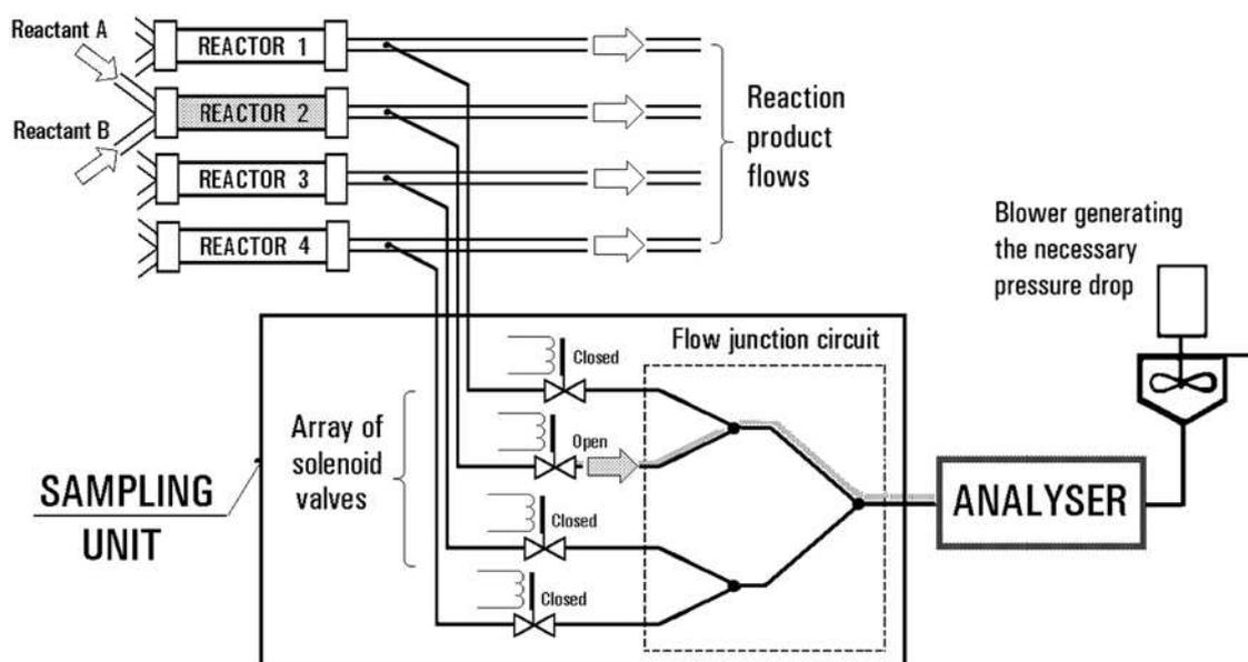
Figure 2. Analysis of reaction products from several mini-reactors sharing a single analyser. This schematic representation shows a mechanical sampling unit, with the flowpaths closed by solenoid valves.
