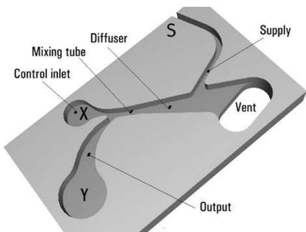
Figure 10. Alternative design of the microfluidic valve with enhanced jet pumping effect. Note (in comparison with Figures 5 and 7) the presence of the full jet pump with mixing tube and a long diffuser.
