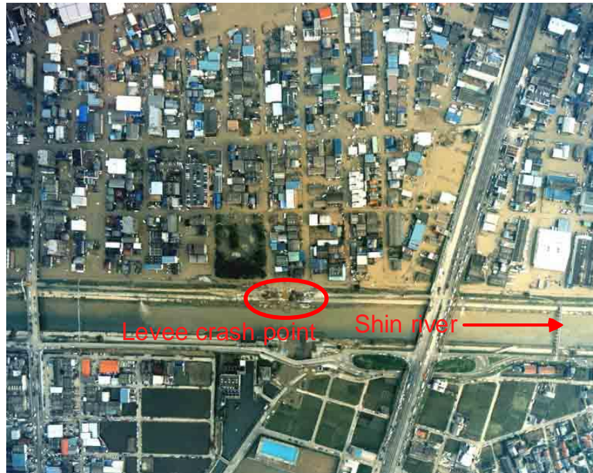
Figure 3 Levee crashing by 2000 Tokai torrential rainfall at Shi n river, September 2000 (Photo is quoted from the website of Kokusai Kougyo Co. Ltd.).
