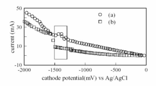
Fig.2 Current-potential relations of (a) a solution containing  $1.33x10^{-2}$  M Bi(NO<sub>3</sub>)<sub>3</sub> and  $1.33x10^{-2}$  M Na<sub>2</sub>EDTA as a complexing agent, and (b) a solution containing  $2x10^{-2}$  M Na<sub>2</sub>S<sub>2</sub>O<sub>3</sub> in a nitric acid solution of 50ml.
