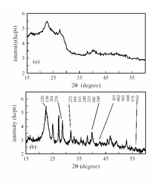
Fig.3 X-ray diffraction patterns of (a) as-deposited  $Bi_2S_3$  and (b)  $Bi_2S_3$  annealed in a flow of argon gas for 0.5hr at 423K. The  $Bi_2S_3$  thin films were electrodeposited from a nitric acid solution of  $4x10^{-2}$  M Na<sub>2</sub>S<sub>2</sub>O<sub>3</sub>,  $6x10^{-3}$  M Bi(NO<sub>3</sub>)<sub>3</sub> and  $6x10^{-3}$  M. The rectangle indicates the diffusion control region.
