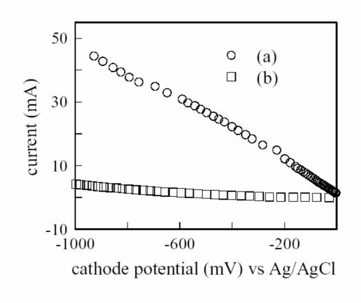
Fig.1 Current-potential relations of (a)  $1.33x10^{-2}$  M Bi(NO<sub>3</sub>)<sub>3</sub> and (b)  $2x10^{-2}$  M Na<sub>2</sub>S<sub>2</sub>O<sub>3</sub> in a nitric acid solution of 50ml. A solution of Na<sub>2</sub>S<sub>2</sub>O<sub>3</sub> was kept still for 24 hr and the top clear solution was used.
