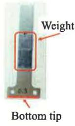
Fig.3.2.2 Shutter-blade model with weight
