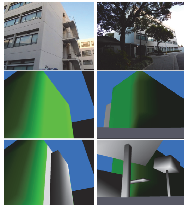
Figure 4.2: The actual conditions (top row), 3D target surfaces are highlighted in green in the initial plan (middle and bottom row) and obstacle primitive models are added (gray surfaces in bottom row).
