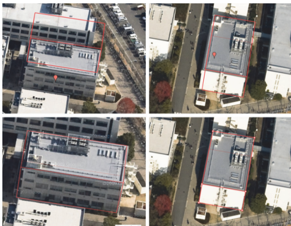
Figure 2.4: Photogrammetry-based modeling process with multiple photos; Building Maker allows adjusting the size and positions of the blocks corners to that of building on the photos.
