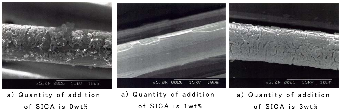
Fig.2-4 The coating layer of the carbon fiber surface made by the coating liquid that changed quantity of addition of SICA
