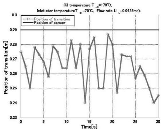
Fig. 6 Fluctuation of transition point (inlet velocity  $0.0425\text{m/s}$ )
