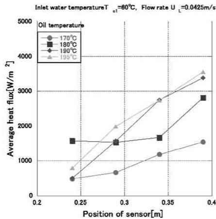
Fig. 12 Average heat flux and position of sensor (inlet velocity 0.0425m/s)
