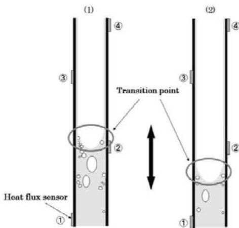
Fig. 3 Flow situation (inlet velocity  $0.0425\text{m/s}$ )
