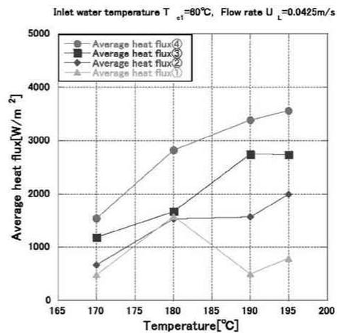
Fig. 10 Average heat flux and inlet oil temperature
