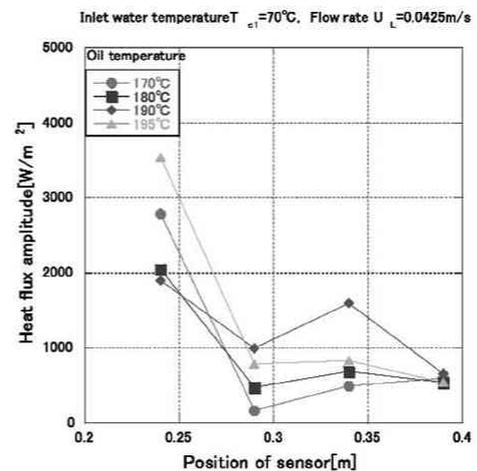
Fig. 19 Heat flux amplitude and position of sensor
