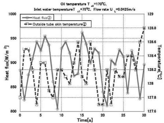
Fig. 4 Fluctuation of heat flux ② and outside surface temperature ② (inlet velocity  $0.0425\text{m/s}$ )
