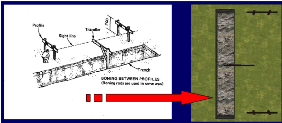
FIG. 5: Visualisation of traveller and sight rails.
