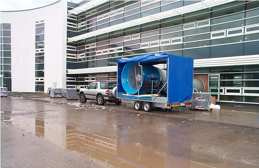
**Figure 1. Air Leakage Testing at Riverside House, January 2003.**
