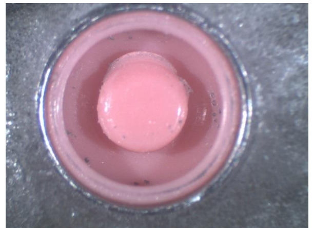
Figure 12: Locator ® male component after 1440 cycle, damage noticed in the internal retention section
