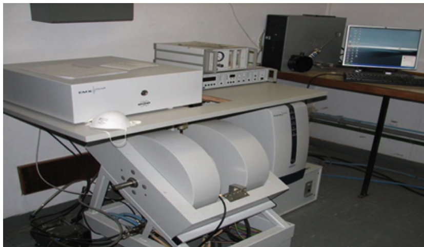
Figure 3.16: Photograph of the ESR apparatus used in this study for OH radical detection
