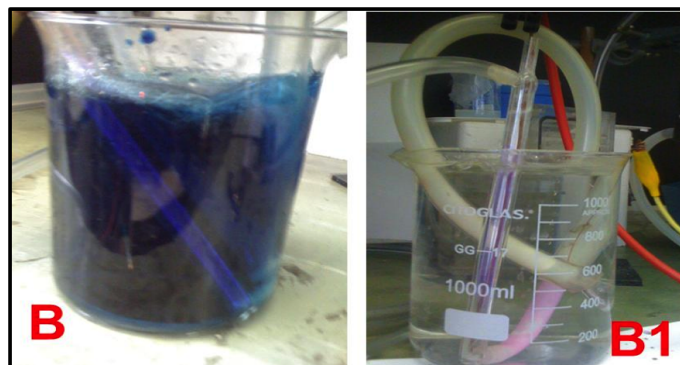
Figure 4.12: (B1) The decoloration of MB after 30 min, using the dissolved ozone from OK-3, UV and other species (B)
