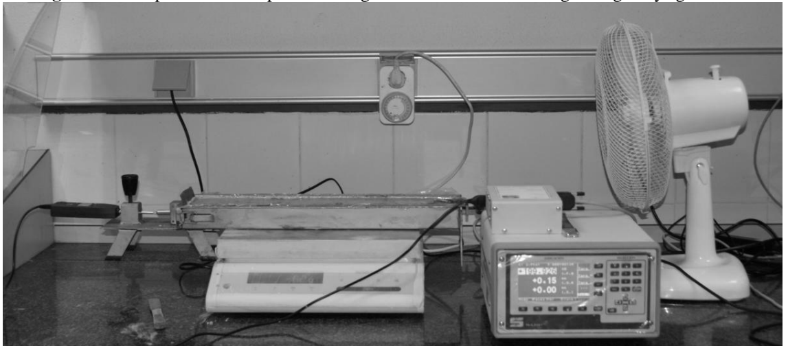
Fig. 2 Experimental setup for shrinkage and mass loss monitoring during early ages
