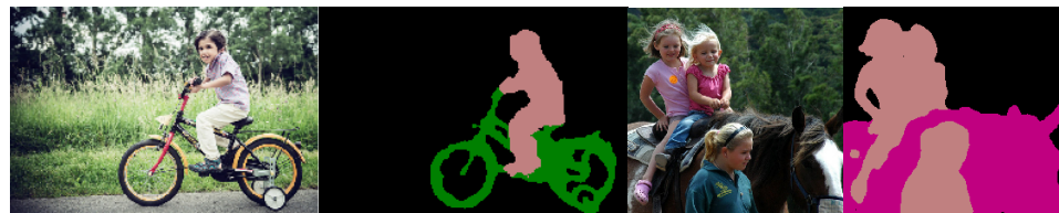
Figure 4. Examples of the image masks from DeepLabv3+. These images come from the Pascal Visual Objects Category dataset. Each color denotes a different class label, with black being background.
