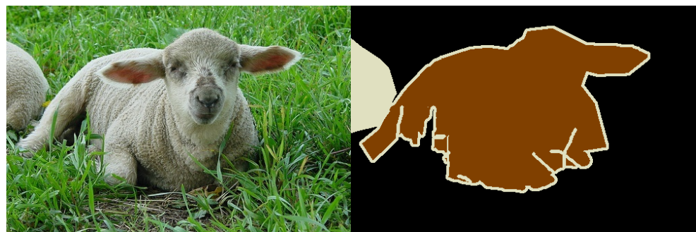
Figure 1. An example of semantic image segmentation taken from the Pascal Visual Object Class dataset. The image on the right is a mask, where each pixel is numbered according to the image class.
