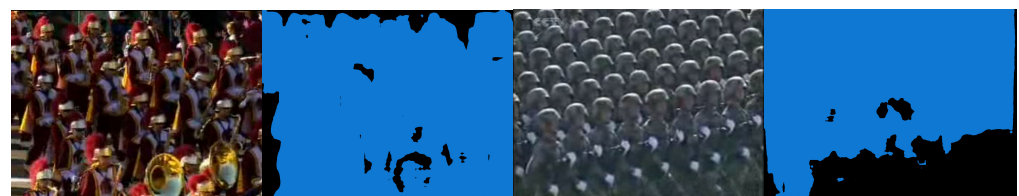
Figure 7. Examples of failure cases from the the UCF101 dataset. The first example is labeled “Marching Band” and the second is labeled “Military Parade”. In both cases, the clutter of same-label objects results in a degenerative blurring filter.
