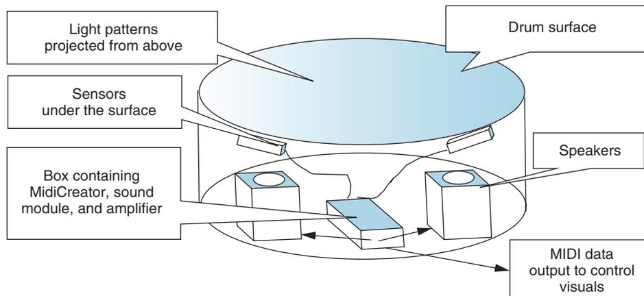
Figure 2. The audiovisual drum concept, shown in cross-section.
