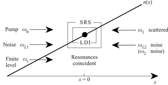
**Figure 1.** The five-wave geometry of the SRS–LD interaction.
