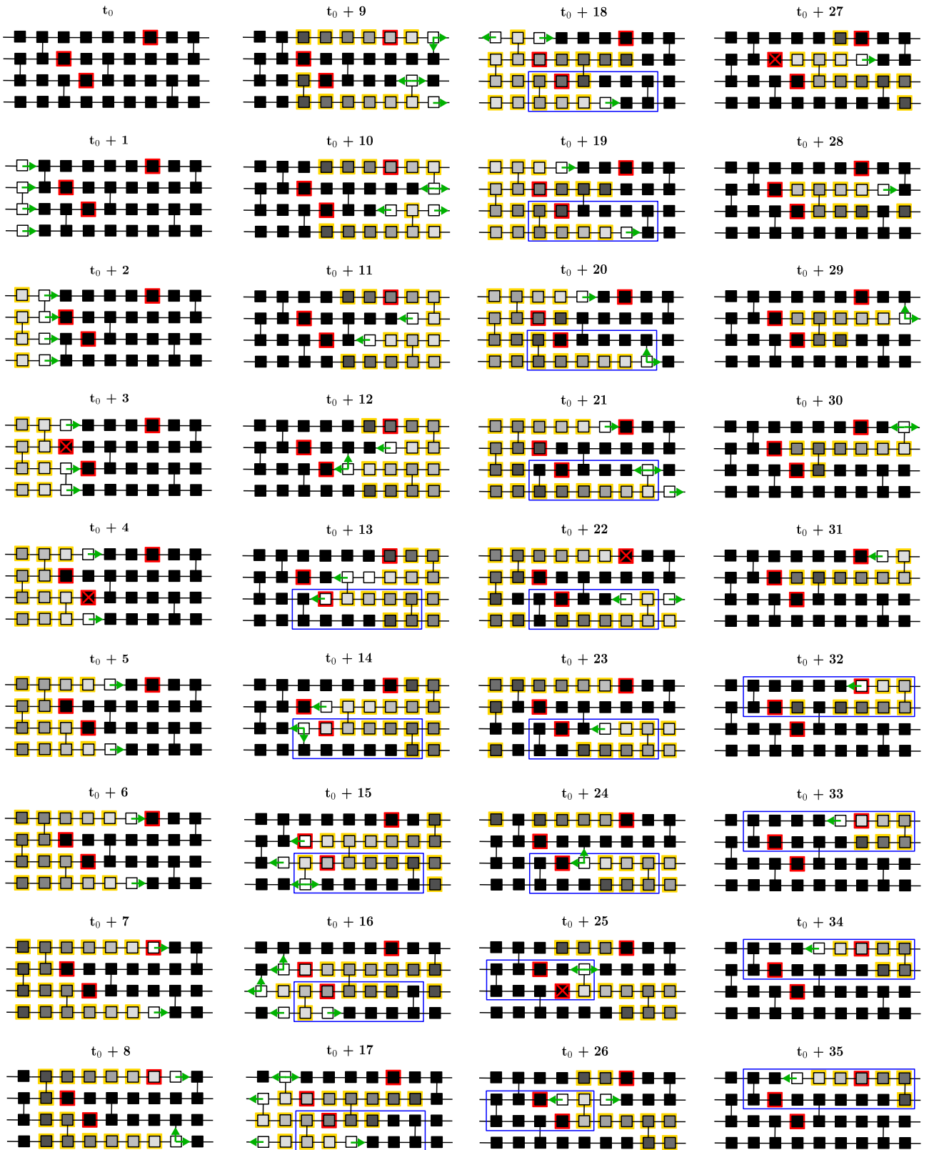
Figure D.12: Sequence of activations of the coupled re-entrant circuits presented in Fig. 3.24. Resting cells are shown in black. Excited cells are shown in white. Refractory cells are shown in grey-scale with a yellow border. Green arrows indicate the movement of the excitation wavefront. Red bordered cells are susceptible to conduction block. A red cross indicates that a cell susceptible to conduction block has failed to activate when prompted to do so by a neighbour. The blue box indicates the region corresponding to an active re-entrant circuit. This figure has been extracted from [20], see appendix B.1 for details about attributions and permissions.
