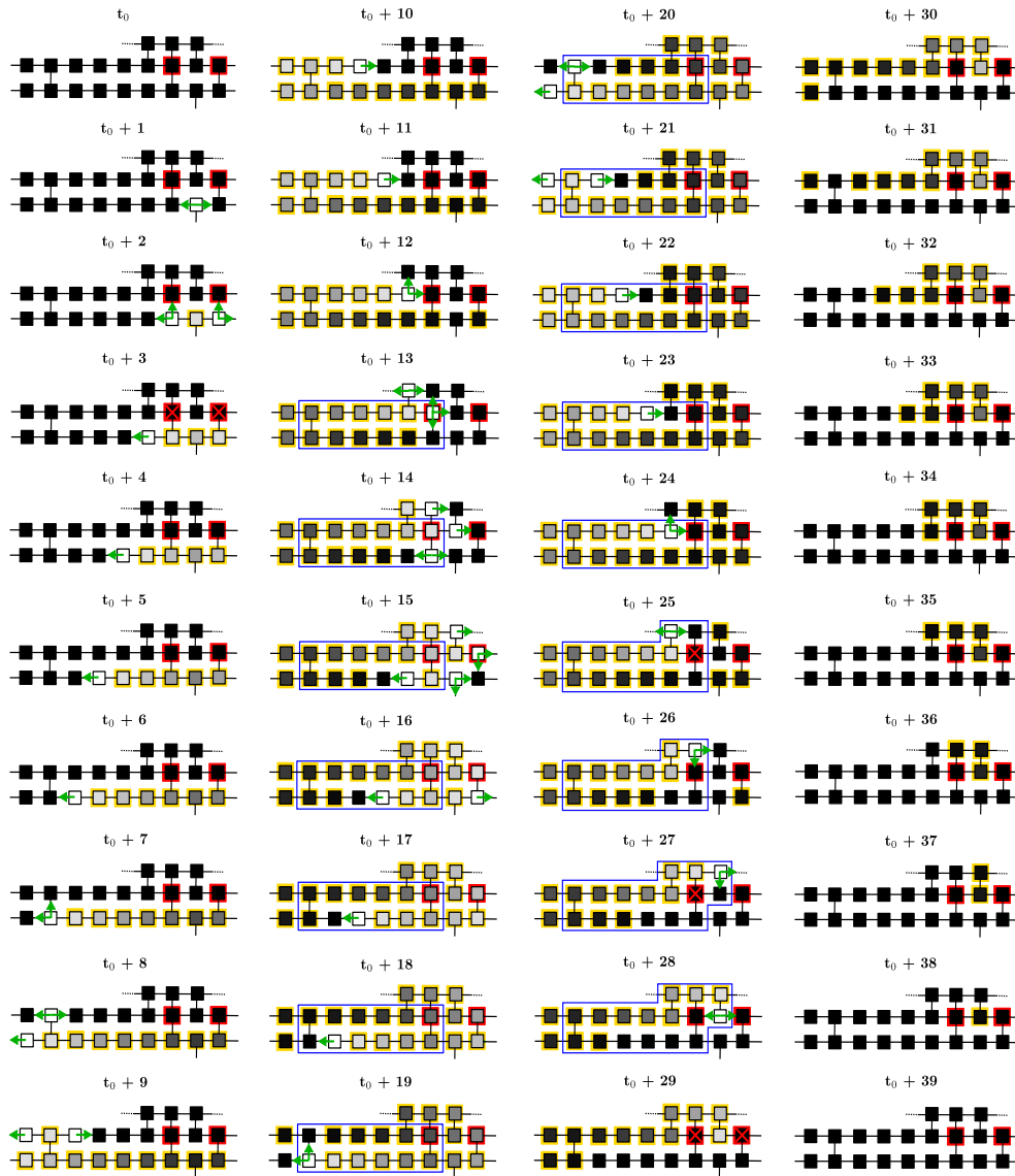
Figure D.11: Activation and deactivation of the complex critical structure presented in Fig. 3.23. Resting cells are shown in black. Excited cells are shown in white. Refractory cells are shown in grey-scale with a yellow border. Green arrows indicate the movement of the excitation wavefront. Red bordered cells are susceptible to conduction block. A red cross indicates that a cell susceptible to conduction block has failed to activate when prompted to do so by a neighbour. The blue box indicates the region corresponding to an active re-entrant circuit. This figure has been extracted from [20], see appendix B.1 for details about attributions and permissions.
