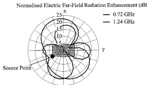
Fig. 8. Radiation patterns of the corner excited sheet.
