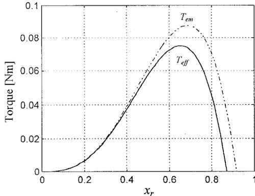
Fig. 2 Torque vs.  $x_r = R_m/R_s$  curves
