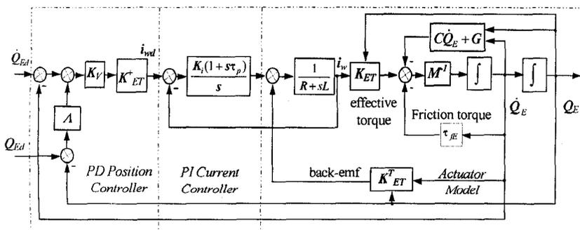
Fig. 4 Block diagram of closed-loop control system
