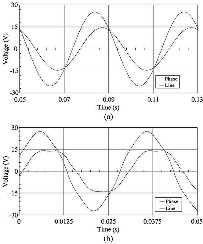
Fig. 4. Back-EMF waveforms. (a) Motor 1. (b) Motor 2.
