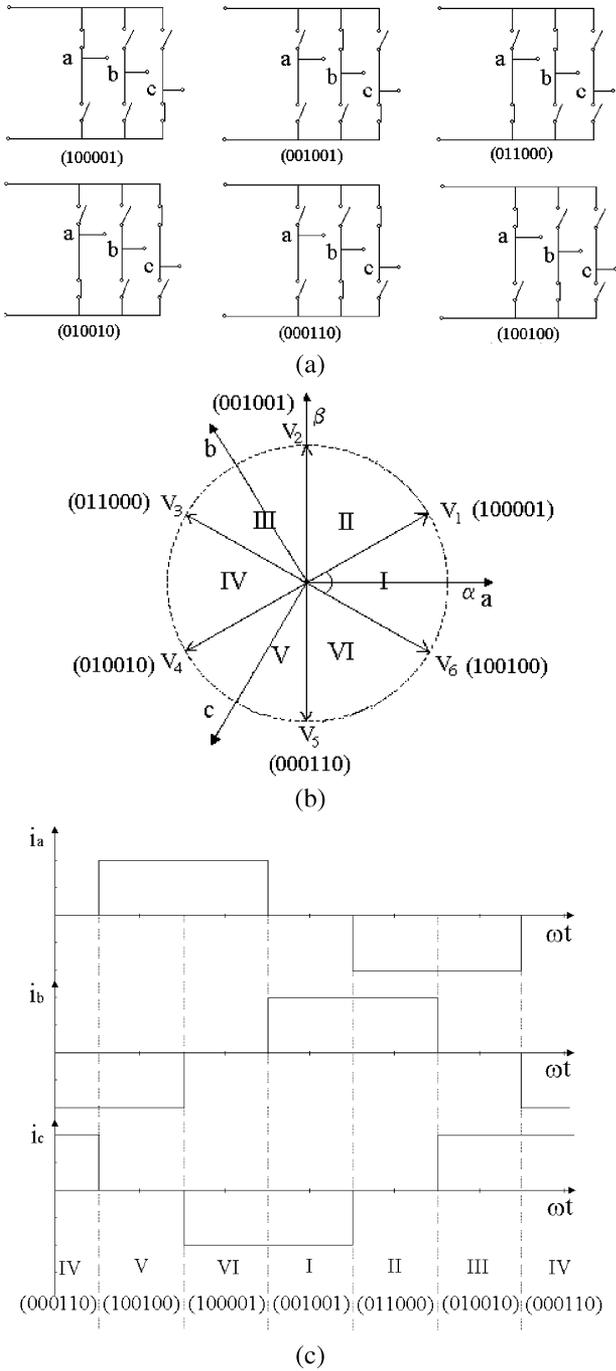
Fig. 1. Nonzero-voltage space vectors for BLDC drive.
