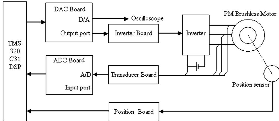
Fig. 6. Schematic of BLDC drive system.
