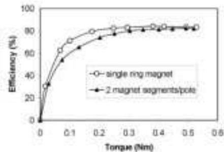
Fig. 8. Measured efficiency–torque characteristics of Halbach magnetized motors.
