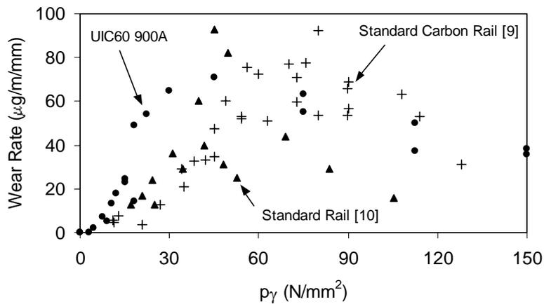
figure 3 Total wheel and rail wear rate in the heavy wear regime
