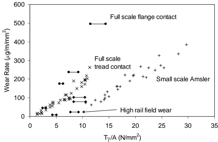
figure 4 Comparison of rail wear data from small and full-scale laboratory tests and the field [11]
