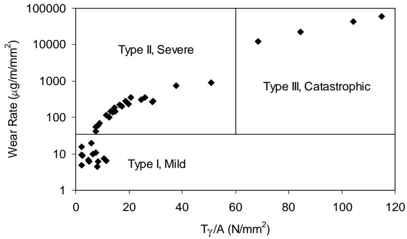
figure 1 Wear regimes identified during twin disc testing of BS11 rail material versus Class D tyre material [5]
