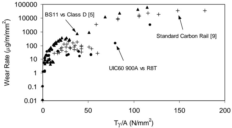
figure 2 Wear rates resulting from twin disc testing for a number of different material combinations
