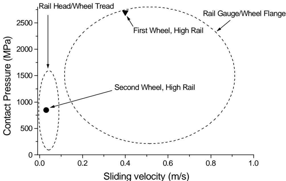
*figure 9* Wheel/rail contact conditions on the Stockholm local railway network derived from GENESYS simulations [6] (also shown are results from Medyna simulations of the Älvsjö test track [16] for the first and second wheelsets)
