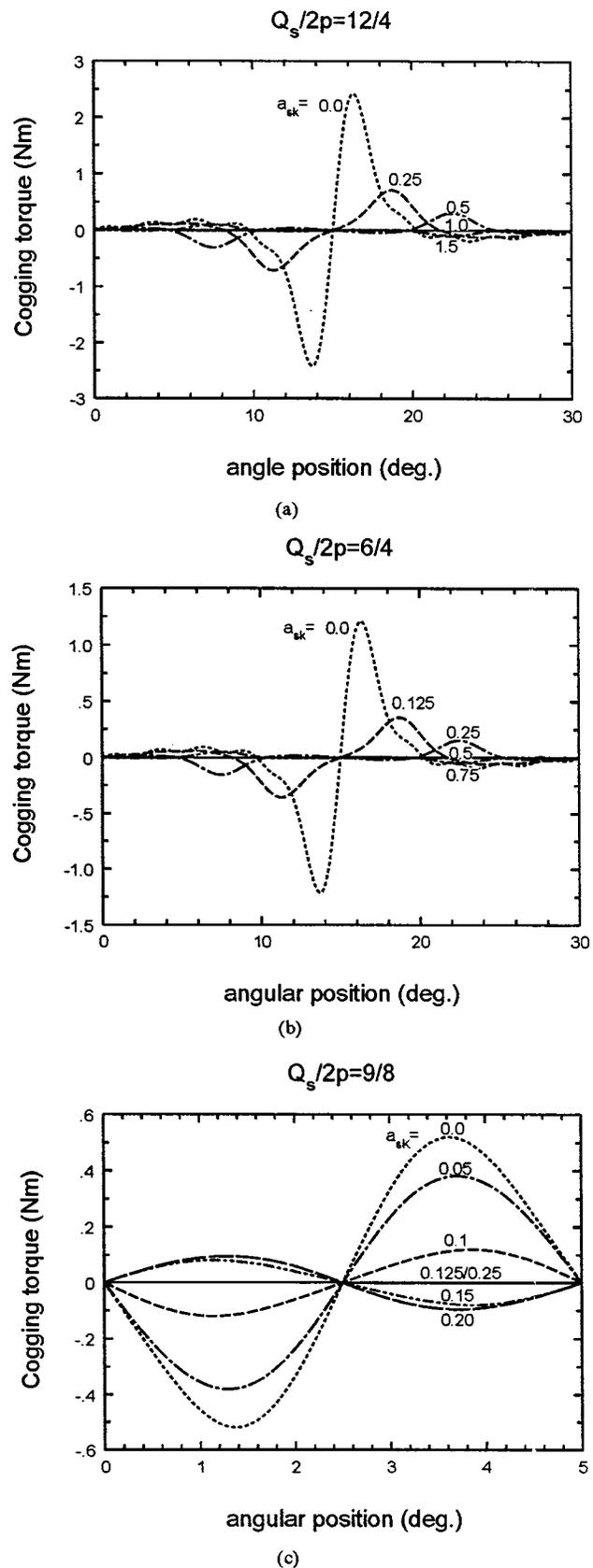
Fig. 11. Effect of skewing on cogging torque waveform.
