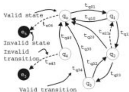
Fig. 1. Definition of valid and invalid states and state transitions for an arbitrary FSM. Normal operation is defined by a valid transition ( $t_{qpc}$ ) between valid states ( $q_x$ ). Faulty operation is defined by an invalid state ( $e_x$ ) or invalid transition ( $t_{e pc}$ ). Note how an invalid transition can also occur between valid states (e.g.,  $t_{e21}$ ) if the transition is not within the system specification.
