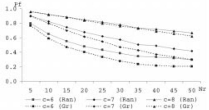
Fig. 10. Comparison of random and greedy detector generator algorithms for variation in failure probability  $P_f$  against the number of tolerance conditions  $N_r$  for match length  $6 \leq c \leq 8$ .
