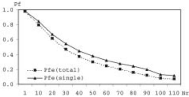
Fig. 13. Failure probability  $P_{fe}$  against the number of tolerance conditions  $N_r$  for total fault detection  $P_{fe}(\text{total})$  and single cycle detectable  $P_{fe}(\text{single})$  faults. Match length  $c = 7$ .
