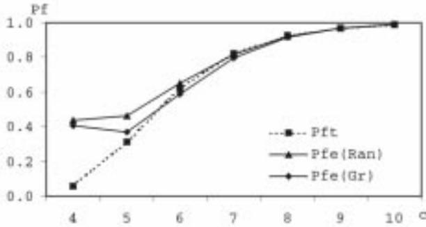
Fig. 9. Theoretical ( $P_{ft}$ ) and experimental ( $P_{fe}$ ) variations in the probability of failing to detect the presence of a fault for  $4 \leq c \leq 10$ ,  $N_r = 10$ . Experimental plots show the random detector generator  $P_{fe}(\text{Ran})$  and the greedy detector generator  $P_{fe}(\text{Gr})$  algorithms applied to the generation of tolerance conditions.
