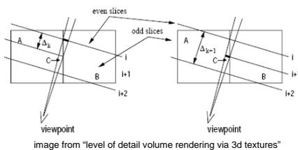
The two pictures figure opacity correction at level transitions for orthographic and perspective views. They depend on whether we look through a brick at the finer level or vice versa.
