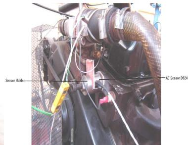
Tests was conducted on a Ford FSD 425 four-cylinder four-stroke, in-line OHV, direct injection diesel engine, rated at 52kW at 2700rpm. AE data is acquired using acoustic emission sensors placed on cylinder head and high speed data acquisition system.
