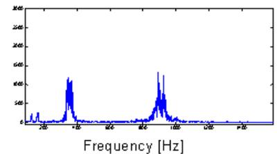
Spectrum of bending vibration
