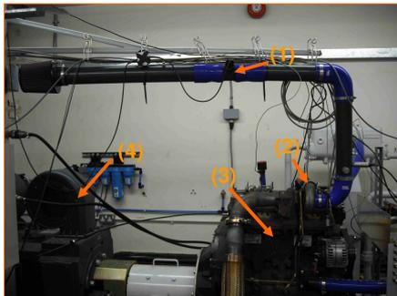
**Left:** Picture shows engine test facility. The labels (1), (2), (3) and (4) show the orientation of the air mass flow meter, the compressor, engine and dynamometer respectively.
