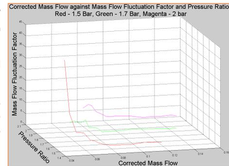
**Right:** To quantify the pressure ratio fluctuation the difference between maximum and minimum pressure ratio was used. This range was then investigated on the graph against both average pressure ratio and average corrected mass flow.
