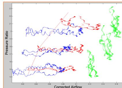
These flows are shown to fluctuate to such a large degree that they cross the surge line even when the average point is well within the heart of the map.
