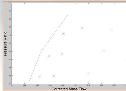
**Left:** Typical points of compressor performance. Red line is the surge line, to the left of this line the compressor goes into surge. Surge is an unstable operating condition observed at low mass flows and can cause severe damage and hence is undesirable
