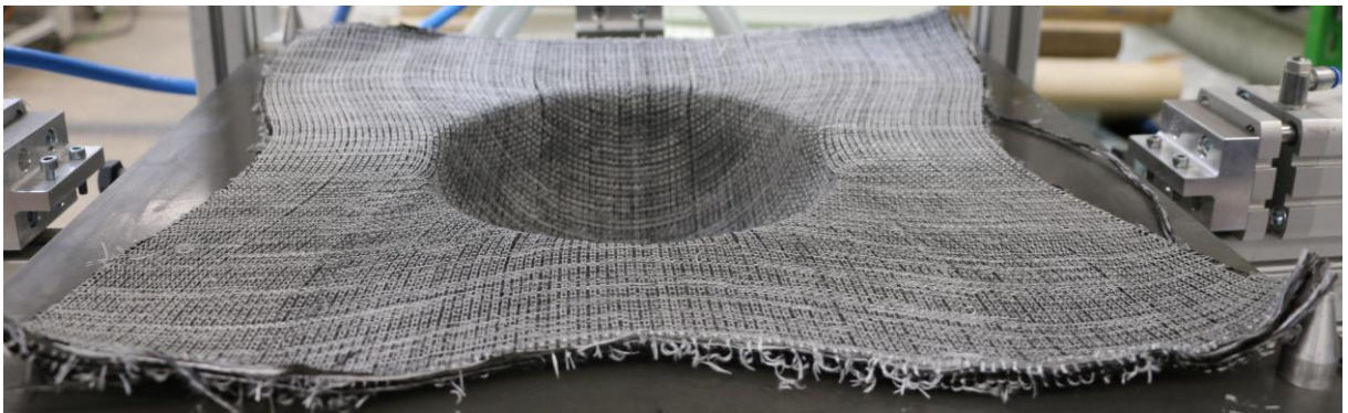
Figure 7-18: 3D preform of BWKF CF/PA 4-layer at 2 bar setting of blank holder pressure (right after forming)
