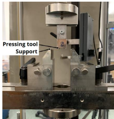
Figure 5-29: Four-point bending test of FRP coupon specimens on Zwick Z100 tensile machine
