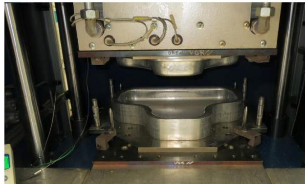
Figure 5-20: CAD model of T-cup shell-like forming tools and the installation of the developed tools on a RUCKS laboratory press at ILK © D. Weck
