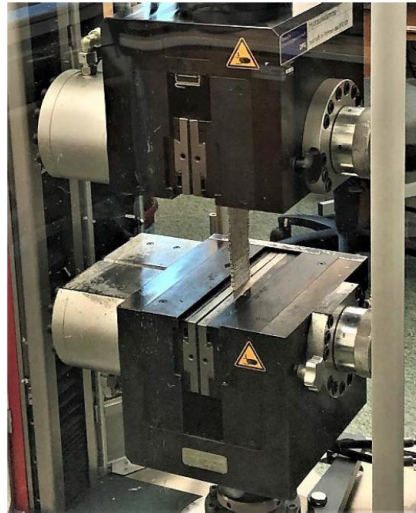
Figure 5-6: Tensile test of BWKF CF/PA 2-layer V1 on a Zwick Z100 machine
