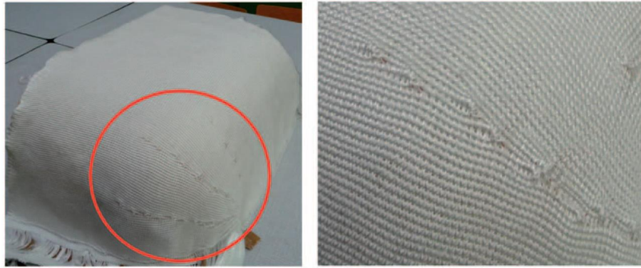
Figure 2-21: 3D complex BWKF preform of a truck corner connection [219]
