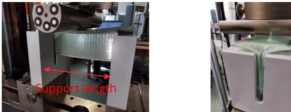
Figure 5-34: Three-point bending tests according to DIN 14125 (method A) of T shaped rib-stiffened FRP
