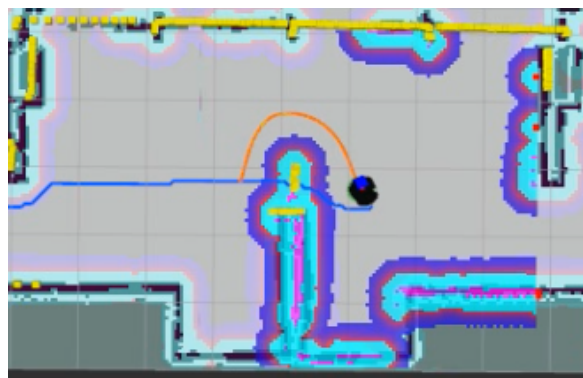
Fig. 1.10 An example path plans visualization (top view). The global plan is coloured in blue and the local plan in orange.
