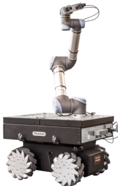
(b) The RB-KAIROS is a completely integrated Collaborative Mobile Manipulator (CMM), designed for the development of industrial tasks [192].
