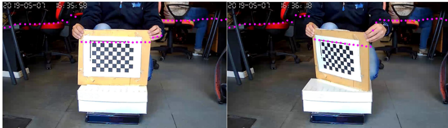
Fig. 2.13 Laser points projected in the image plane.
