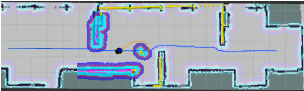
Fig. 2.25 Test scenario 3: OSGP algorithm reaction to a generic obstacle detection.
