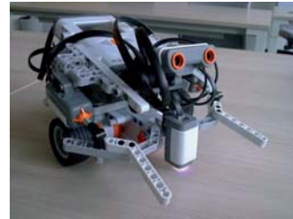
Figure 2: The Mindstorms class robot. It is equipped with a color, ultrasonic and two touch sensors.
