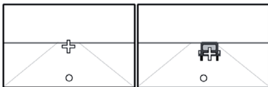
Fig. 5: Near and far points for a straight road with a vanishing point and a road segment with a lead car.
