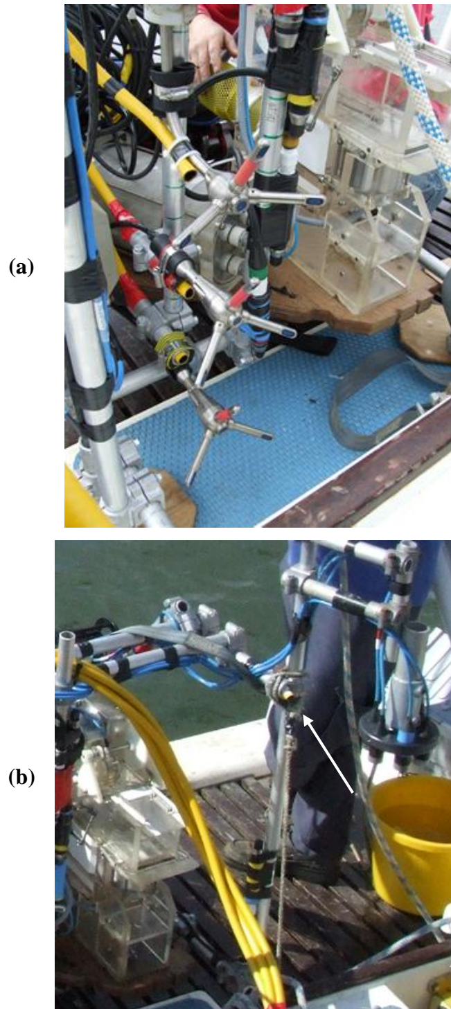
Figure 3 – Photos showing locations of the pump sample inlets on the instrument frame, with (a) three inlets, one positioned behind each ADV, and (b) one inlet located 7 cm above and 20 cm behind the ABS transducers.
