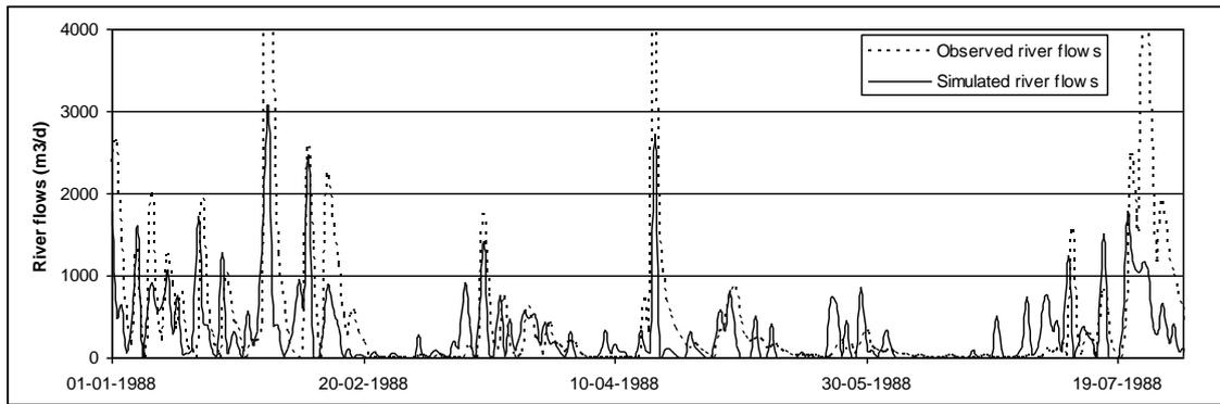
**Fig. 2** Calculated versus simulated overland flows. Run-off coefficient values retrieved from files.
