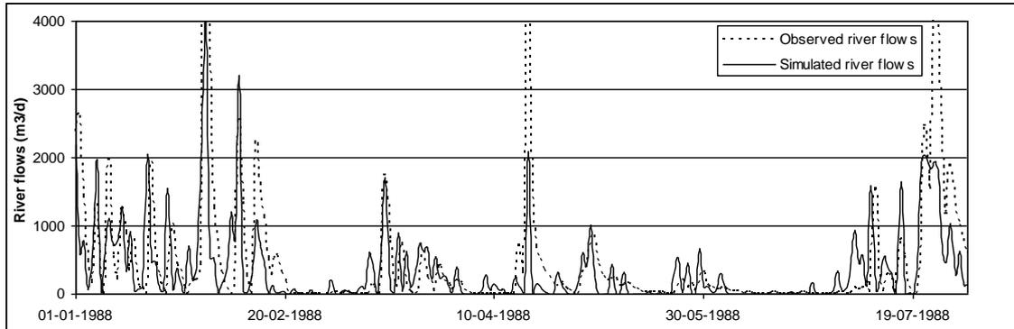
**Fig 3** Calculated versus simulated overland flows. Run-off coefficient values related to topographical gradient and SMD values.
