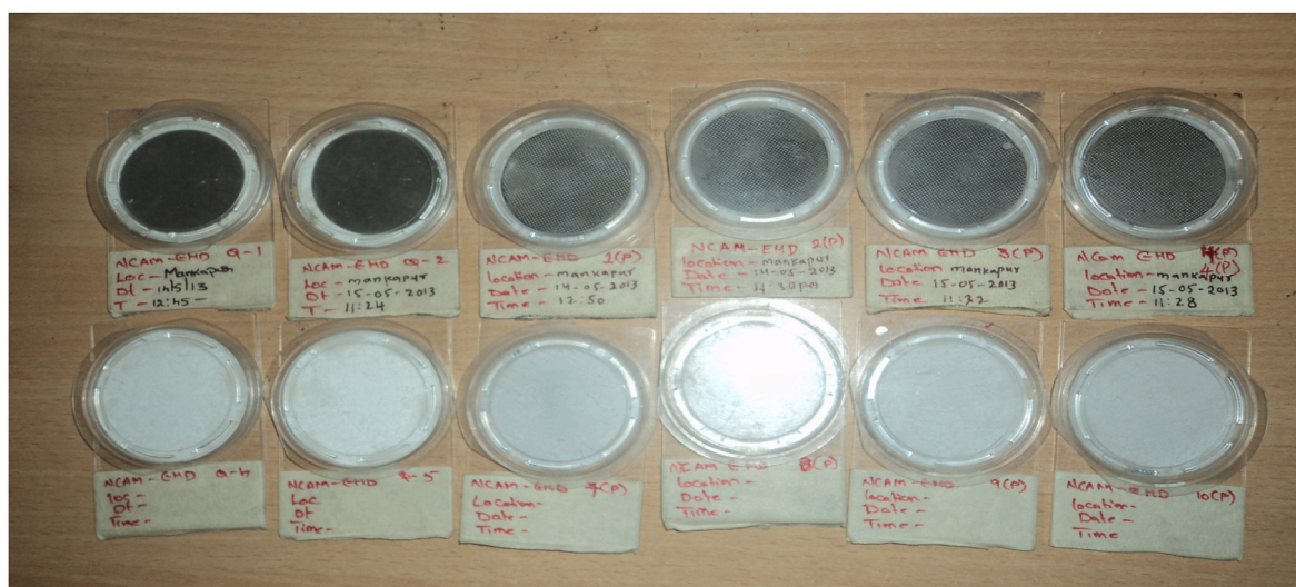
Fig. 7. Top: 24-hr samples of PM 2.5 (first two from left) and PM 10 (last four from left) from an urban area in Nagpur district during summer; bottom: blank filters.
