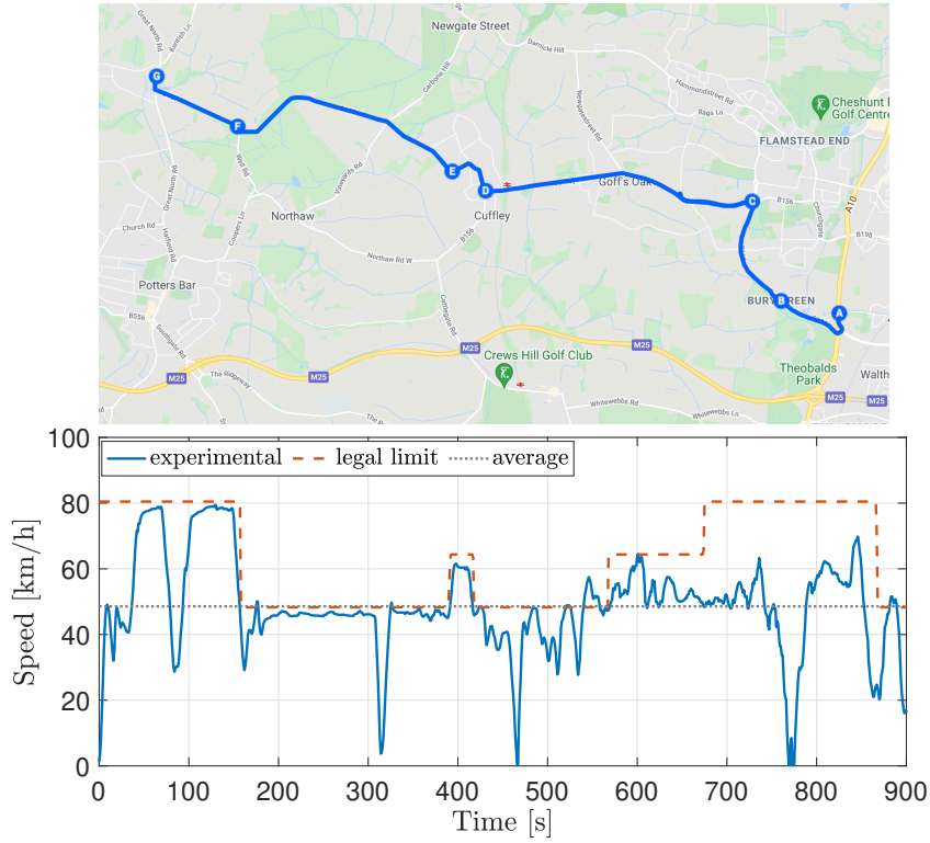
Fig. 4.8 Top: 12.1km rural route selected as a real-world vehicle driving mission https://t.ly/n2wL . Bottom: Experimental driving speed profile for the mission above.
