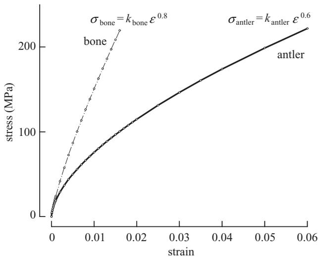
Figure 5. Nonlinear elastic stress–strain curves for normal bone and antler bone produced by using equation (A 1) and constants for bone:  $k_{\text{bone}} = 6.0$  GPa,  $n = 0.8$ ; and for antler:  $k_{\text{antler}} = 1.2$  GPa,  $n_{\text{antler}} = 0.6$ .
