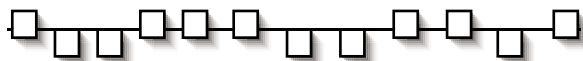
Fig. 10.4. Wall detection. Even when a surface is relatively smooth, sensor readings will rarely lineup perfectly. The straight line represents the wall being sensed. The boxes represent laser readings. Factors such as alignment, sensor error, small outcroppings, etc. all impact what is detected.
