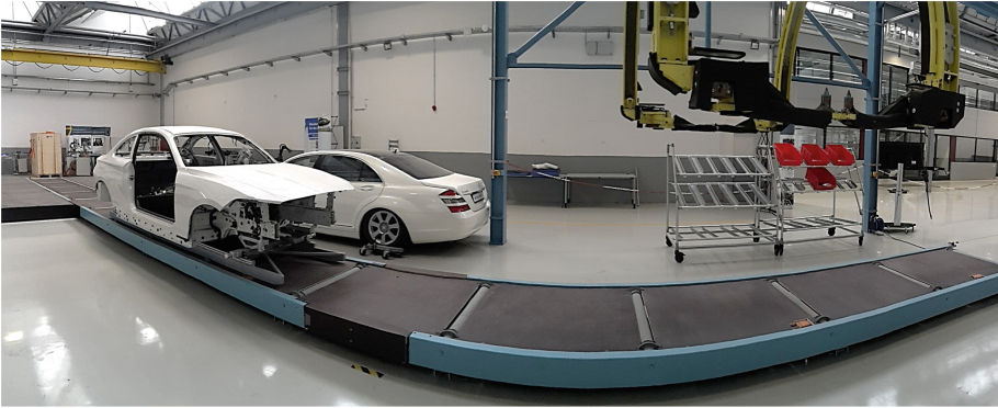
Fig. 8. Skid conveyor system at ZeMA.
