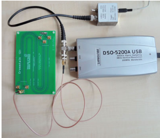
Fig. 18. Home-made time domain reflectometer with scope and generator (Shown with Crosstalk Experiment Board).
