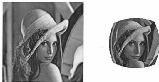
Fig. 4. Foveated image in Cartesian coordinates (left) and curvilinear coordinates (right) [14]
