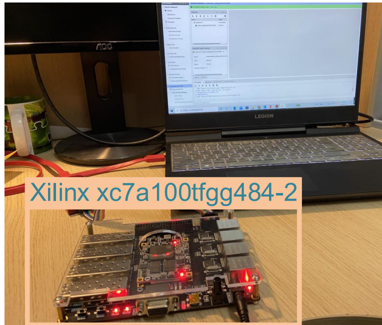
Figure 4.18: Implementat the accelerator on the Xilinx Artix-7 XC7A100T FPGA.
