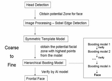
Fig.3 Frontal Facial Detection Model: For individual boosting model, it contains ten base classifiers generated by C4.5 decision tree. The concept of symmetric template model is derived from the symmetric patterns of human face.
